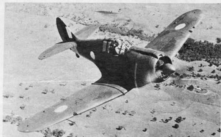
Swept-back wing and stubby fuselage distinguish Australian Boomerang. Fin and rudder and tailplane are rounded on trailing edge.
